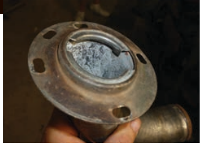
Above, one fuel filler pipe has the fuel cap locking ring formed as part of the pipe. Below, this pipe has a separate cap locking ring. You'll need at least two locking rings, one will remain in the existing mounting hole in the tail panel, and the other will be used on the fuel filler pipe to be mounted to the fuel tank and located in the trunk.
