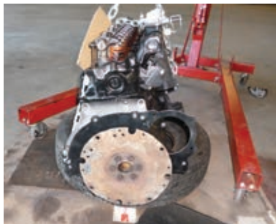
Note the two upper sets of transmission mounting holes. C4s use the lower set as shown; manual transmissions use the upper set.
