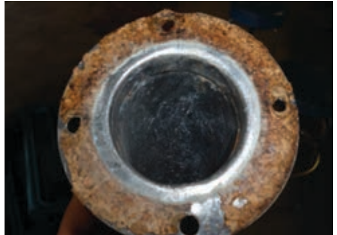
Above, one fuel filler pipe has the fuel cap locking ring formed as part of the pipe. Below, this pipe has a separate cap locking ring. You'll need at least two locking rings, one will remain in the existing mounting hole in the tail panel, and the other will be used on the fuel filler pipe to be mounted to the fuel tank and located in the trunk.
