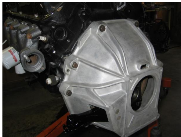
The flywheel, clutch and bell housing were installed while the engine was hanging.
