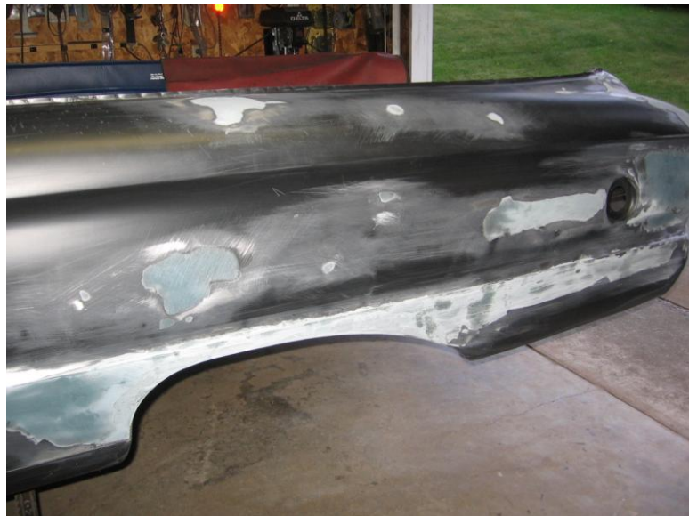
Short kitty hair filler has been applied and sanded.
