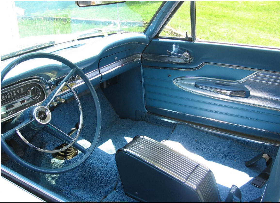
The interior is mostly complete in this picture. The bucket seats are still missing; the window cranks have been installed.
