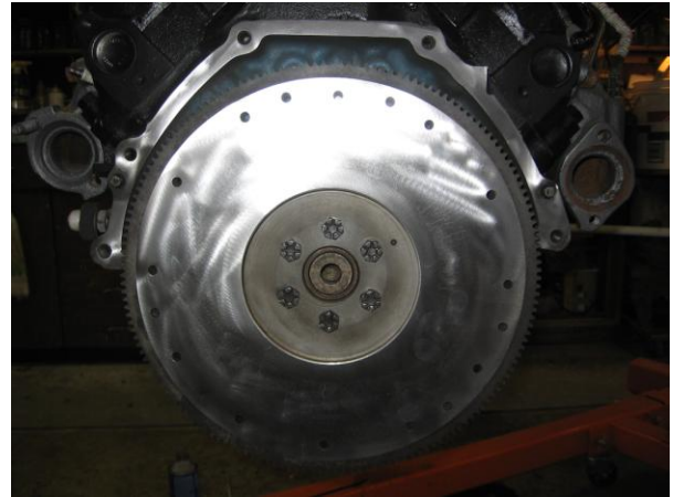
The flywheel bolted and torqued in place.
