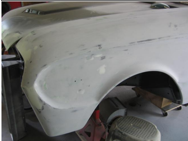
Guide coat sanded off. The dark spots are either the base primer showing through or the guide coat sitting below the level body surface. The lighter shade is filler.
