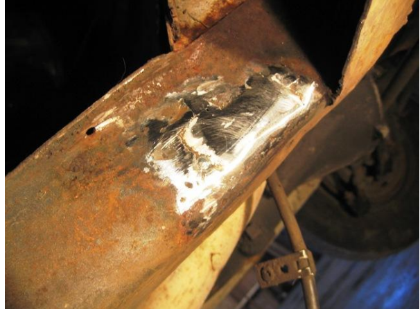
The frame rail is repaired prior to patching the torque box.
