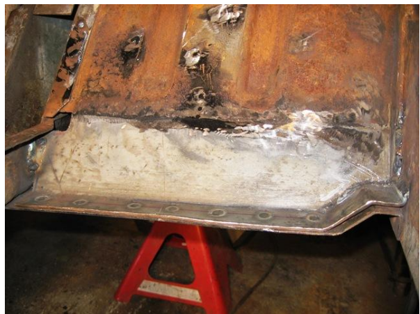
The back side of the torque box is repaired; the toe board patch is next.
