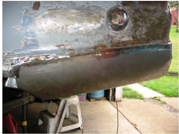
Lower quarter panel patch is welded into place.
