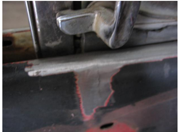
The inner door panel crack is welded shut. The vent window was re-inserted to check the fit around the repair.
