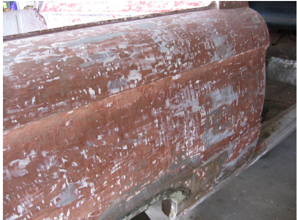
The right rear quarter after multiple coats of stripper and scraping. The original red oxide primer indicates it is almost totally stripped.
