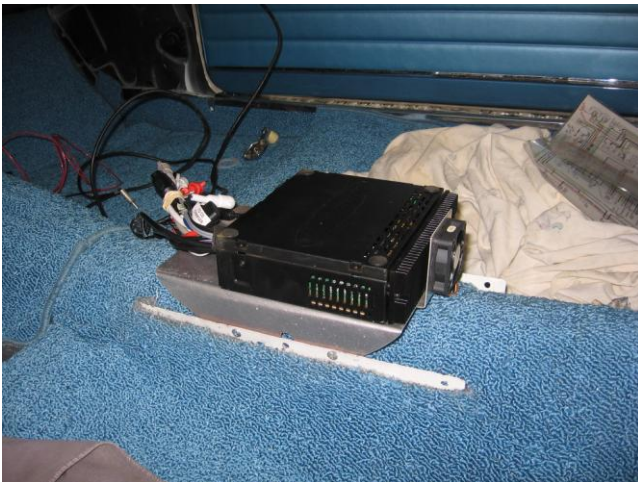
The hidden audio system is mounted to a sheet of aluminum which is then fastened to the console mounts. Notice the small fan at the right of the unit that will help keep the electronics cool.
