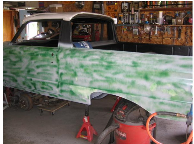
Guide coat applied.
