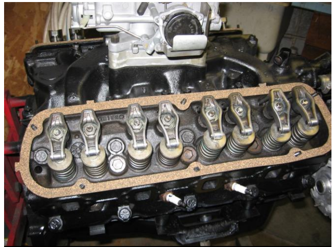
Roller tipped rockers will reduce the friction and also cause less wear in the valve guides.
