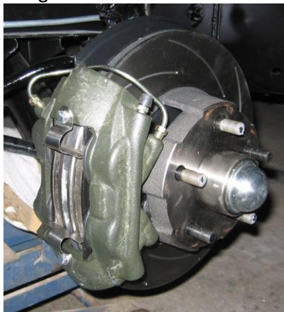
Two views of the completed front disc brake assemblies, notice the rotors are even slotted.
