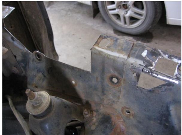
The reinforcement plate is removed and the rusted inner fender material is cut out with a 4" cut off wheel in a pneumatic grinder.
