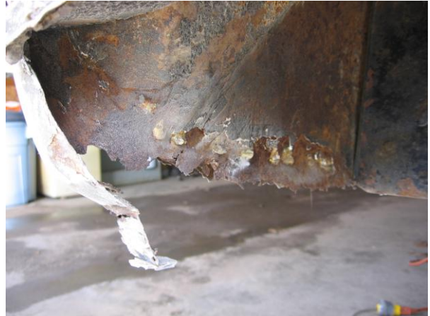
This is a view looking at the back side of the left rear quarter. If you look close, you can see the brazing puddles left
