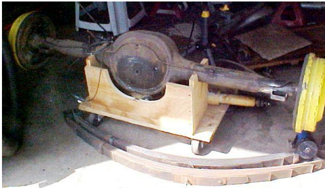
Two views of the axle sitting on the home made dolly. This saves the back and also provides a platform to make any repairs.
