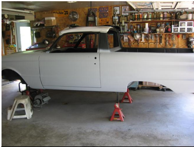
Three heavy coats of high-build primer have been applied.
