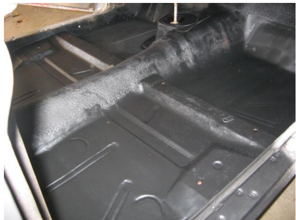
All the floor pans finished and coated with epoxy primer.
