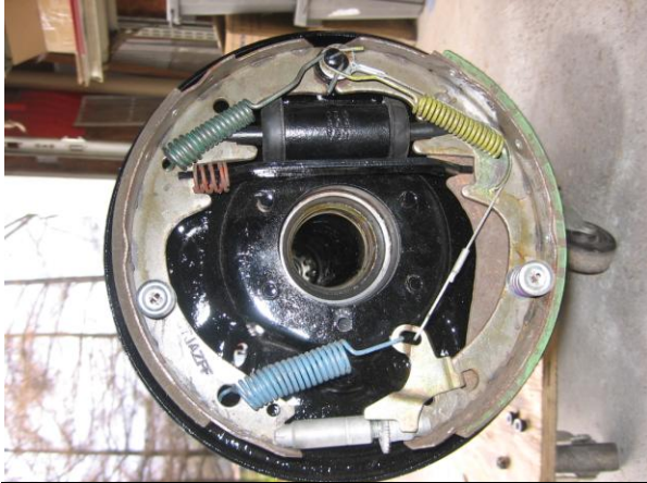
The brake shoes and hardware were in like new condition. Clean it up and put it back together.
