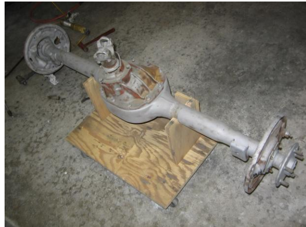
The axle freshly sand blasted waiting for disassembly and a new coating of paint.
