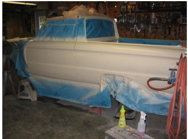
The doors and rear quarters were finish sprayed at the same time. Notice the additional masking.
