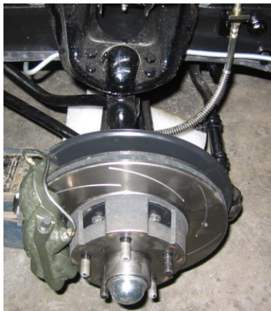
Two views of the completed front disc brake assemblies, notice the rotors are even slotted.
