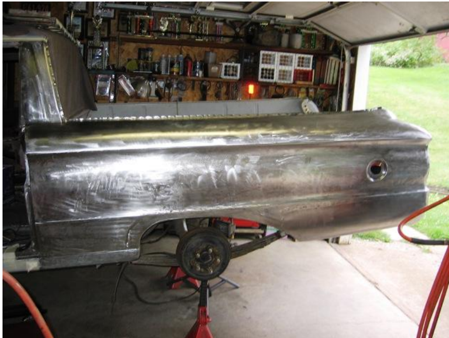
The lower quarter panel patch is clamped in place using vice-grips and seam spacers. A series of 3/8" long welds are placed about 4" apart. This is to reduce heat build-up that may warp a panel.
