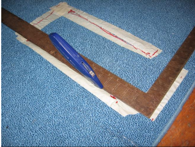
Masking tape, a sharp utility knife and a straight edge are used to cut slots in the carpet for the center console.
