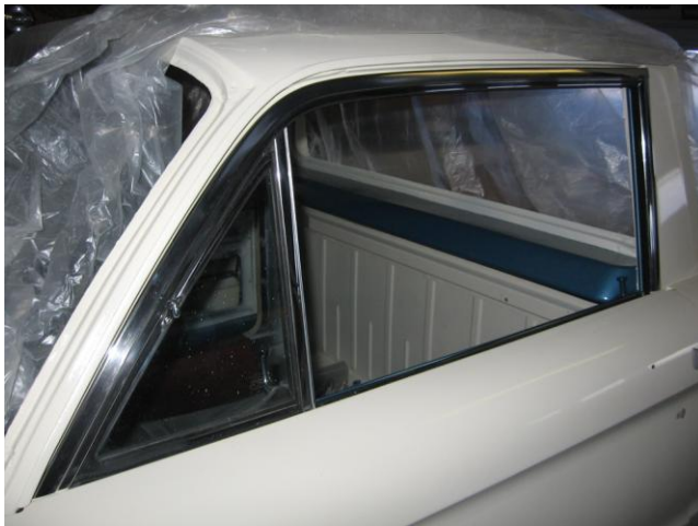
Deluxe window trim installed around door glass.
