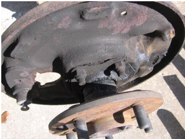
The grease seal is history! Much easier to replace while it is on the cart than on the Ranchero!
