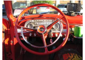
Answer to last month's teaser: The uniqueness is the steering wheel; Tom removed 2" of diameter changing the wheel from the stock 15" to a more modern 13" steering wheel. Tom took photos of the process and it will appear in a future issue.
