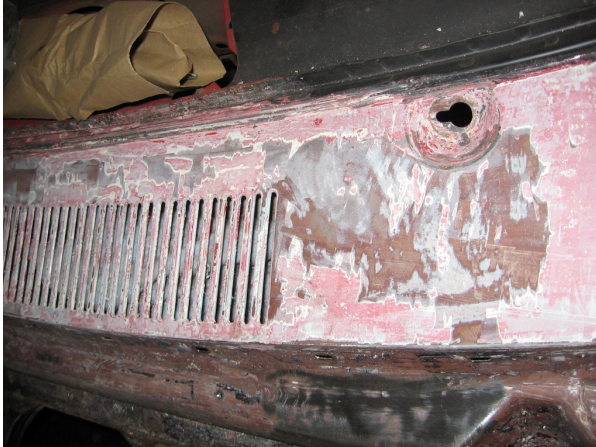
This is a view of the cowl after the first coat of stripper was applied and then scrapped off.
