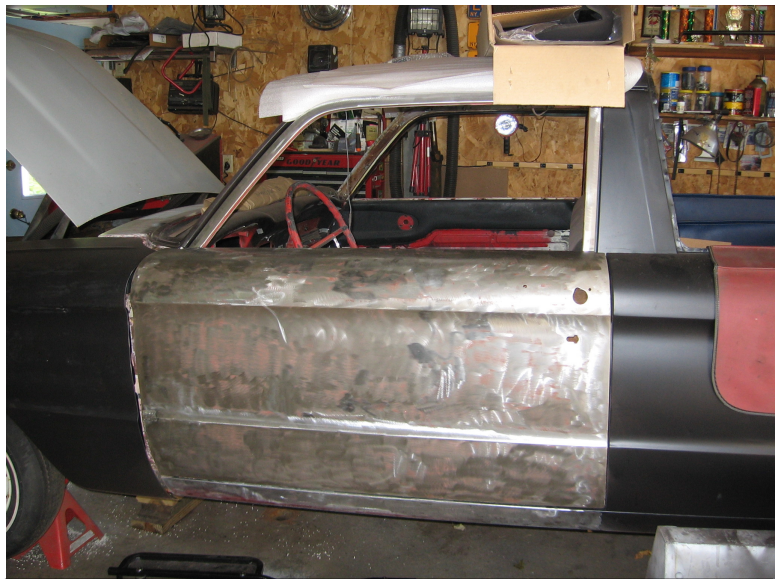
The driver's door chemically stripped, but not sanded. Notice that the rear quarter and the front fender are already stripped and primed.
