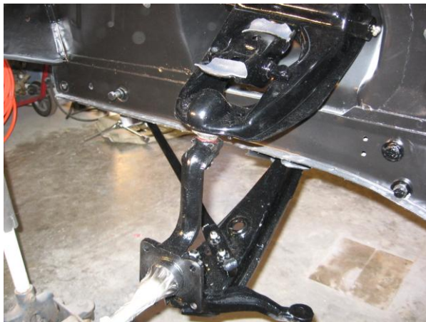
The upper control arm, lower control arm and the strut rod install first.
