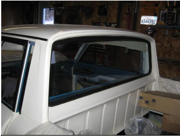
The back window was extremely difficult as its design required installation from the inside.
