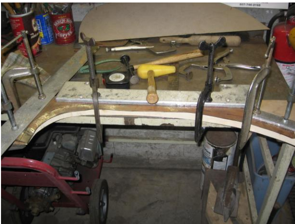
The wooden buck and a piece of sheet metal are clamped to the work bench. The yellow plastic mallet is the tool for hammering with. The cardboard wheel well template can be seen in the background.
