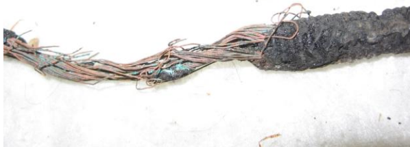
The taillight harness that got melted, this was over the left rear wheel well.
