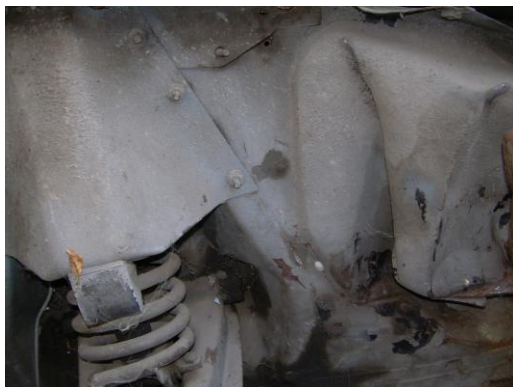
Inner fender damage
