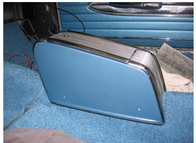
The console hides the unit. There is a lot of wiring running under the carpet, so a lot of pre-planning is required. There is still plenty of room above the audio system for storage.
