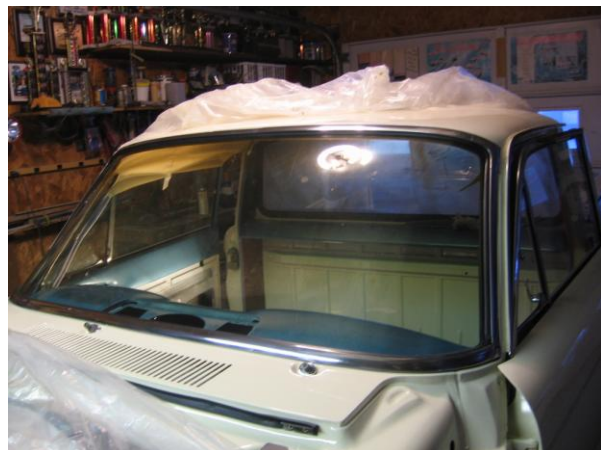
The windshield was installed before the hood and front fenders were for obvious reason.
