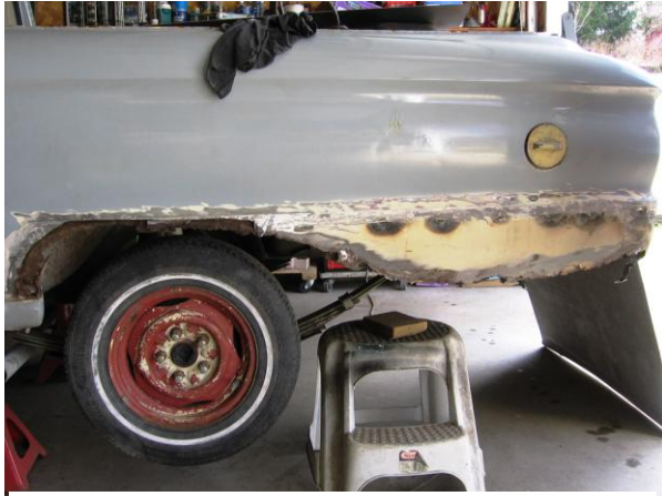
Rear view of left rear quarter after the Bondo and overlapped metal patch was removed. The original paint was underneath the patch.
