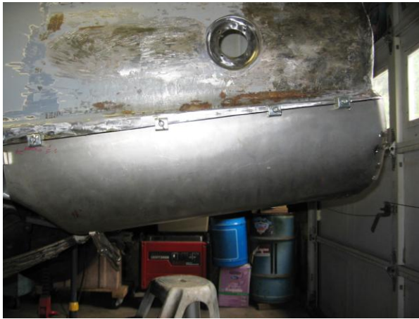
The lower quarter panel patch is clamped in place using vice-grips and seam spacers. A series of 3/8" long welds are placed about 4" apart. This is to reduce heat build-up that may warp a panel.
