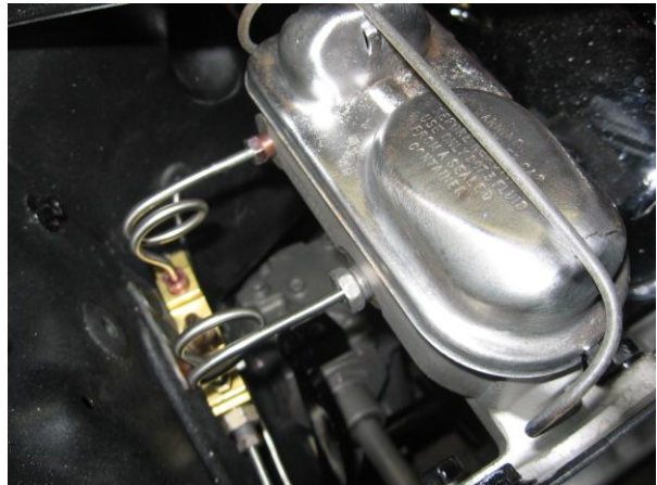
Two views of the master cylinder, notice the loops in the brake lines going from the master cylinder to the distribution block. The loops serve two purposes: 1. they make it easier to tweak the alignment and 2. they allow some flex to minimize stress at the fittings.
