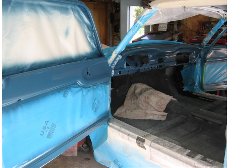
The interior blue finish coat was applied before the final two exterior coats. Notice all the additional masking to keep blue off of the white.
