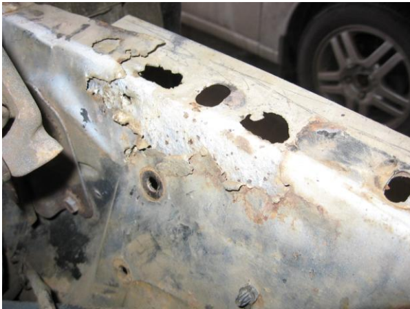
Typical inner fender rust. Notice the inner fender and the reinforcement plate underneath. Both will get patched.
