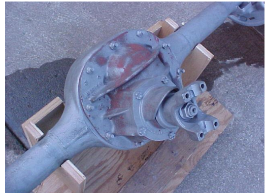
Two views of the axle sitting on the home made dolly. This saves the back and also provides a platform to make any repairs.
